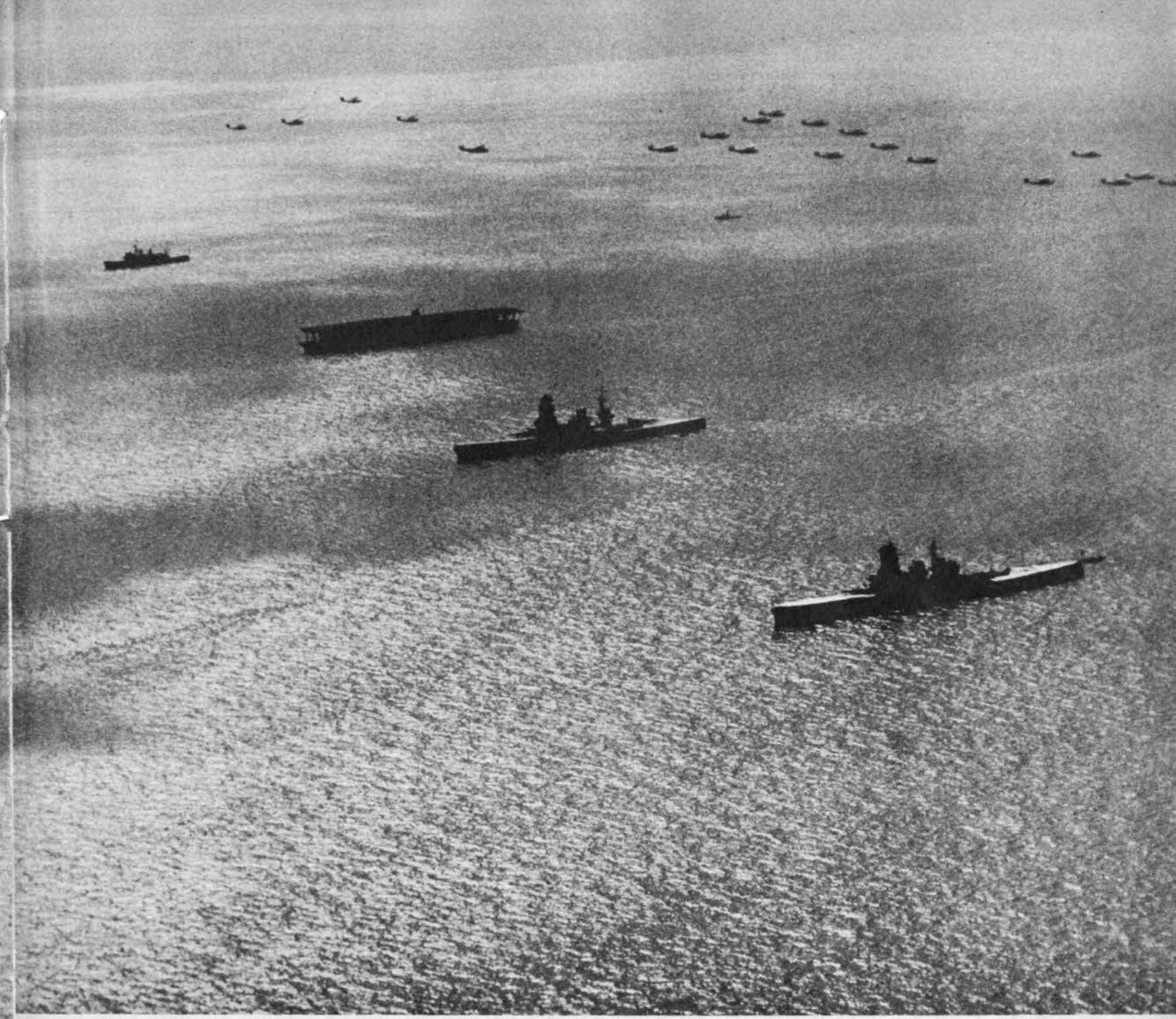
is clearly outlined. In the foreground are two of her four Kongo Class BB's; behind them, two Nagatos. The CV's Hiryu and Akagi (sunk at Midway) are in background, while overhead are Mavis. Tall masts, open superstructure would immediately mark the BB's as Japanese.
